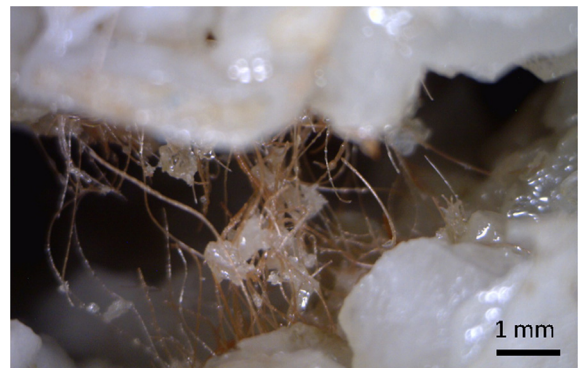
Fig. 10. Crack bridging action of a carpet waste particle.
